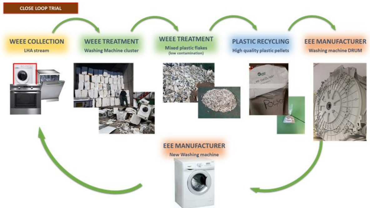
Figure 11 PolyCE close loop demonstrator: from end of life washing machine cluster to new washing machine drum
