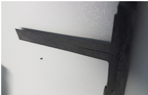
FIGURE 5: BROKEN INJECTION MOULDED SPECIMEN SAMPLE 2
