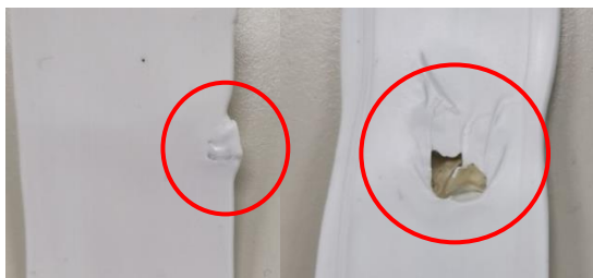
FIGURE 11: CONTAMINATION FLAKE SAMPLE DURING EXTRUSION
