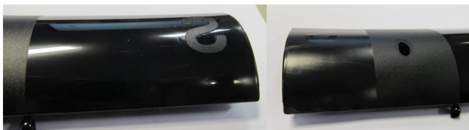
Figure 9: PC moulding trial 2 – extreme drying conditions
