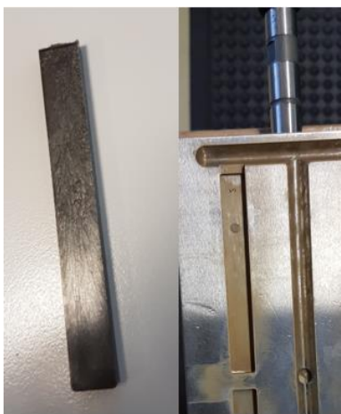
FIGURE 3: LEFT: IMPACT SAMPLE; RIGHT: CORROSION OF TOOL
