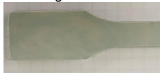
FIGURE 12: COLOUR CLOUDS IN INJECTION MOULDING SAMPLE FROM FLAKES
