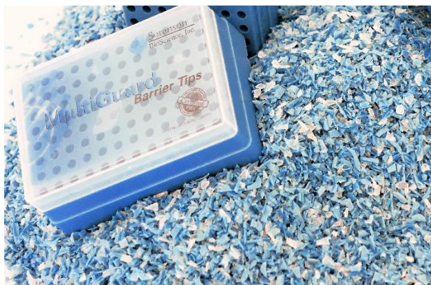
FIGURE 13: PP FROM LAB WASTE: THE WASTE PRODUCT AND THE RESULTING SHREDDED PLASTICS
