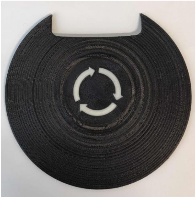
Figure 6A - Demonstrator realized in Post-Consumer PC/ABS (black) and virgin ABS (white) using a Prusa MK3s with MMU2S multi-material unit with a layer thickness of 0.3mm.
