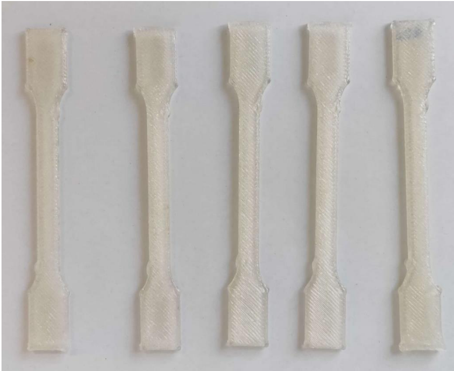
Figure 2A – Tensile bars ISO 527 Type 1A made in TPU using the micro-extruder additive manufacturing 3D printer developed at CPMT.
