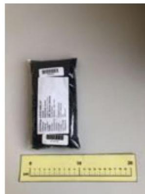
**Figure 25. ABS produced from the plastic flakes coming from the treatment of vacuum cleaners cluster**
