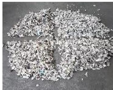
**Figure 9. Output plastic flakes from the washing machines pre-treatment**
