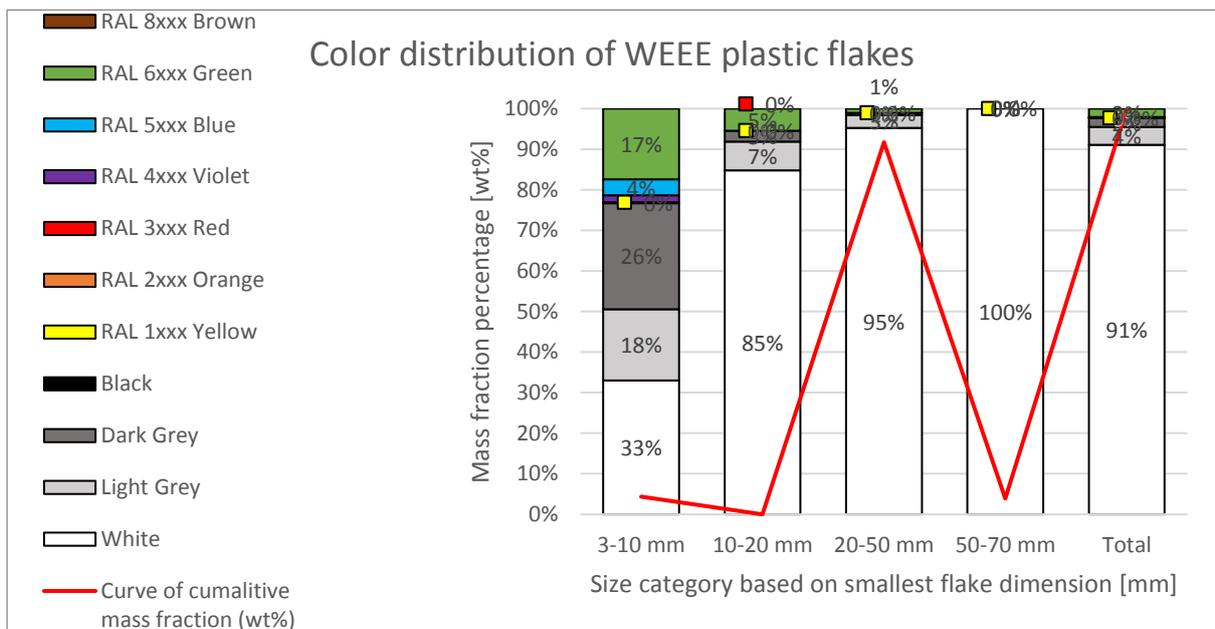
The colour composition of the flakes was dominated by white and light grey shades. A minor content of grey and transparent pieces in the sample was observed visually and is expected to cause the dark grey colour in the composition. The green is expected to come from the conveyor belt as no green pieces could be observed.
