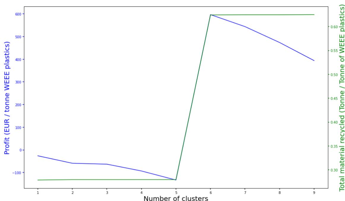
Figure 29. Profits and recycling rates per unit tonnage of recycled WEEE plastics (distributed as in the collected WEEE plastics stream in the EU) when applying optimal clustering strategies for various numbers of clusters.
