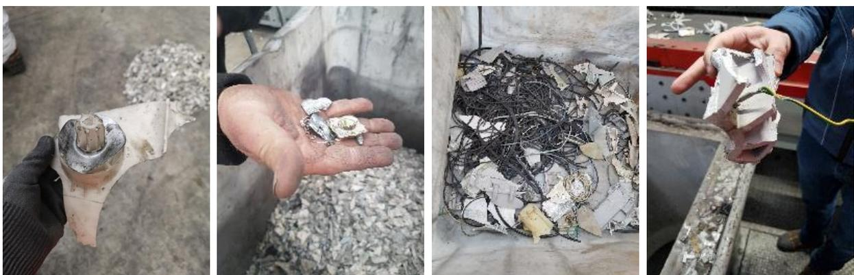
Figure 12. Drums cluster: parts manually removed from the plastic flow
