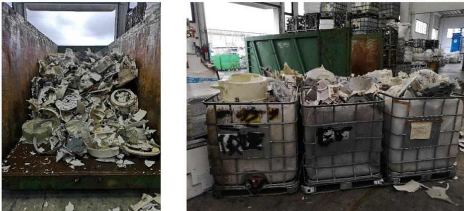
Figure 11. Drums cluster: drums manually dismantled.
