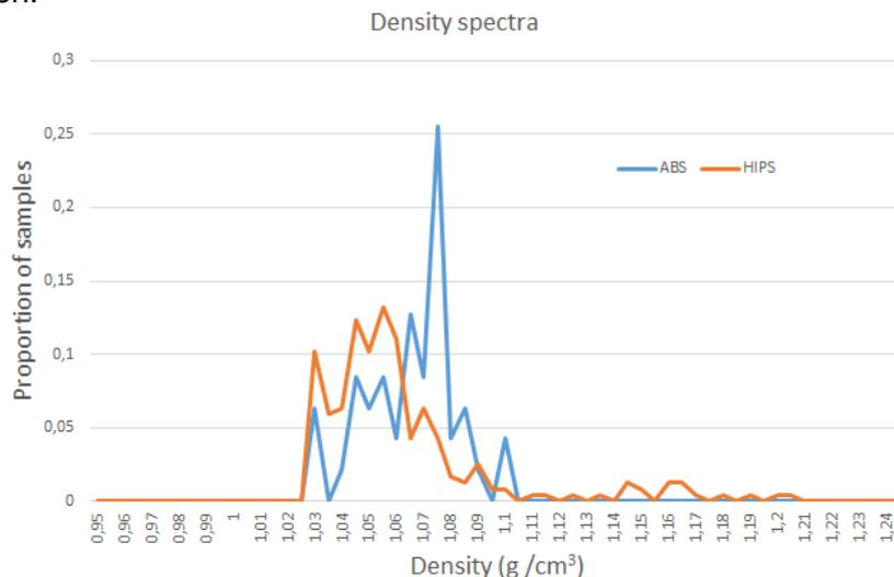
Figure 27. Density spectra of ABS and HIPS
