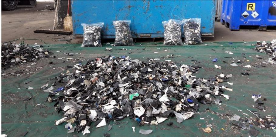
Figure 18. SHA cluster: coffee machines, output material
