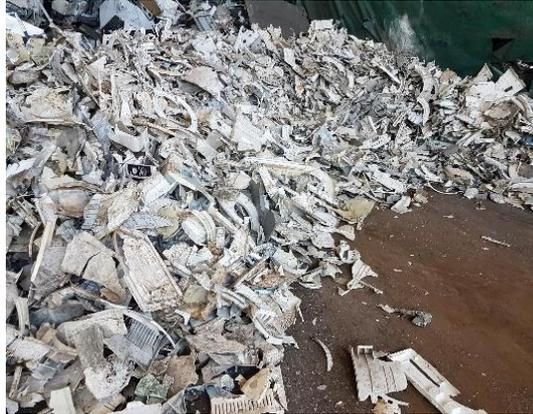
Figure 10. Plastic fractions obtained from the pre-treatment activities performed in Seveso Recupero.
