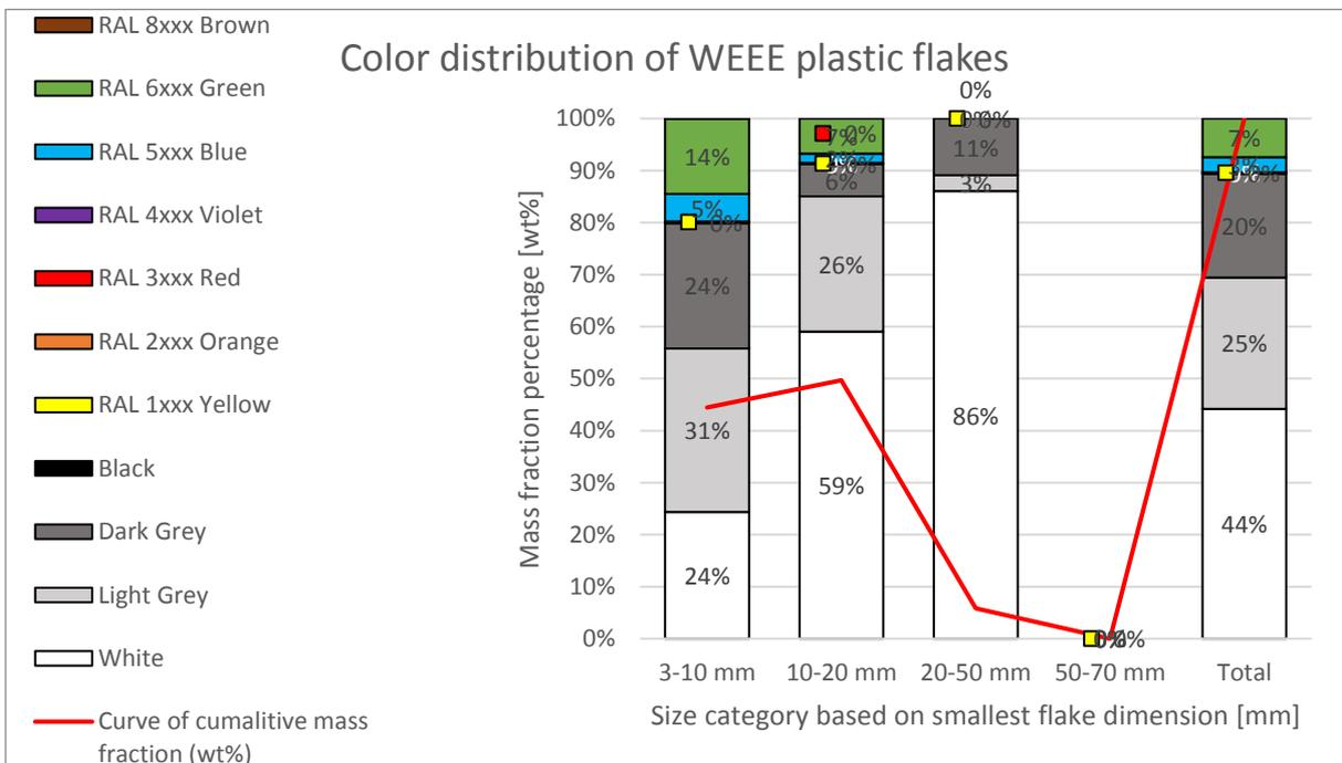
The colour composition of the sample consists of various shades of white, grey and dark grey. Blue and green flakes could also be observed in the sample and confirmed visually. However, the relative amount of 14 % of green colour shades in the 3-10 mm category is expected to
