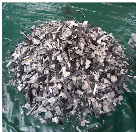
Figure 15. SHA cluster: printers, output material
