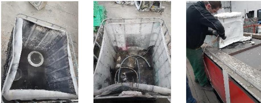
Figure 6. Washing machines cluster treatment: first removal step
