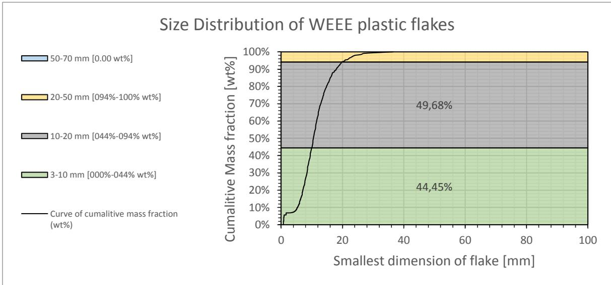
The size distribution of the plastic flakes from fridges is characterized by relatively small flake sizes due to the processing of the plastics in a blade shredder. The fines content smaller than 3mm was tested by sieving and resulted in 1,9 wt%.
