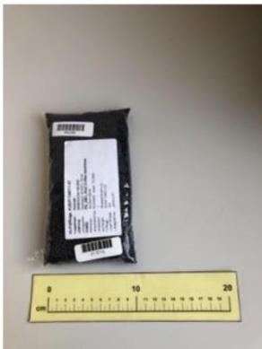
**Figure 26. PC/ABS produced from the plastic flakes coming from the treatment of professional coffee machines cluster**
