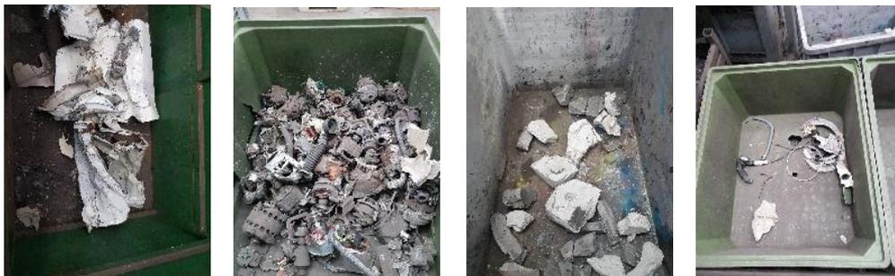
Figure 7. Washing machines cluster treatment: second removal step
