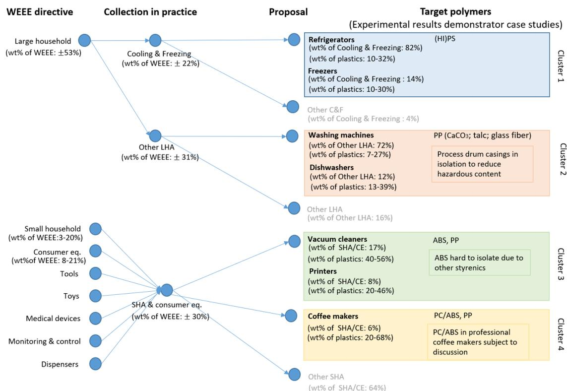
Figure 28. Clustering approach based on the collected data. Weight percentages as indicated are based on [22-34].
