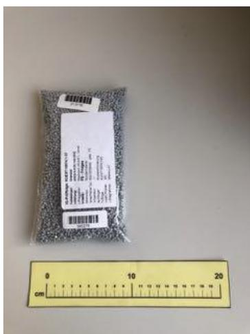
Figure 23. PS produced from the plastic flakes coming from the treatment of fridges drawers cluster
