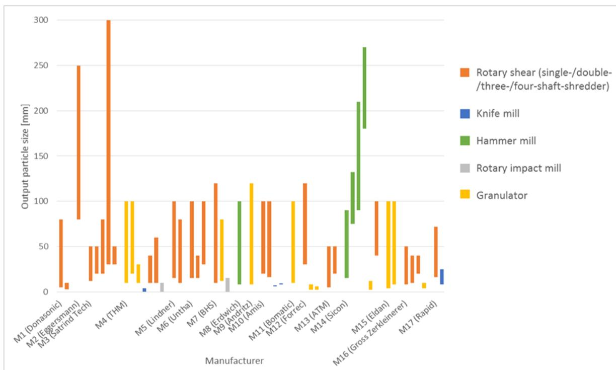
Figure 9: Output particle sizes produced by different shredding technologies
