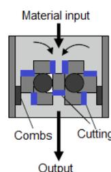
(4) Rotary shear (shredder)
