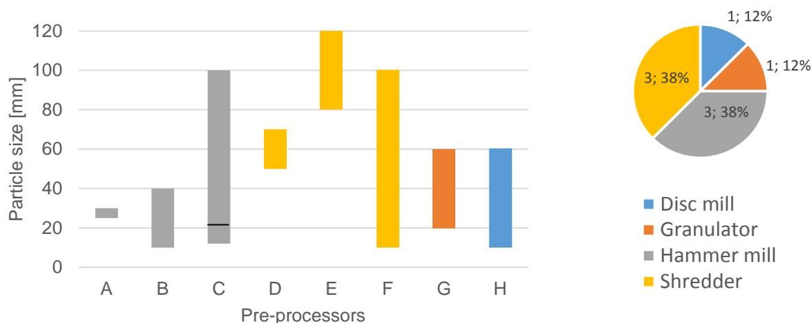
**Figure 10: Particle size of the output plastics fractions from sWEEE treatment (left) and related size reduction technologies (right)**
