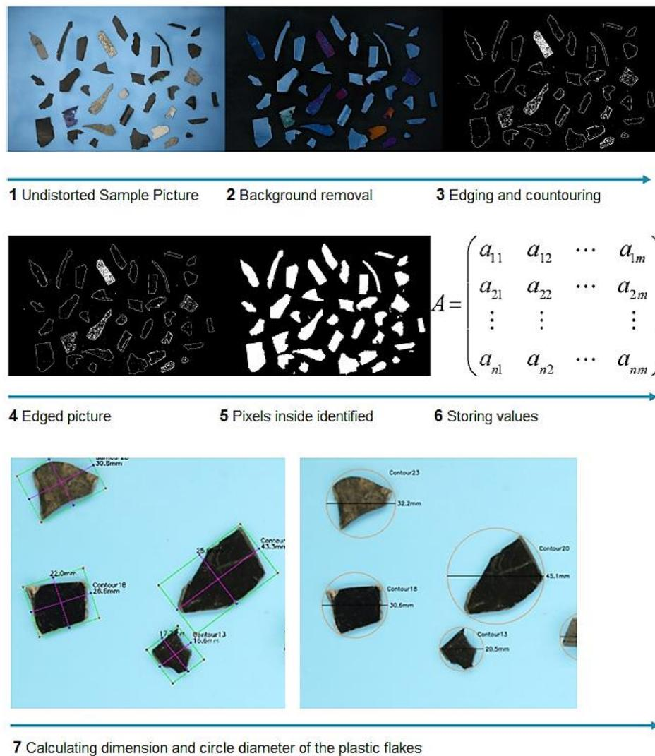
**Figure 8: Flowchart of the identification of the plastic flakes with the computer vision system (Antico & Beerten, 2018)**
