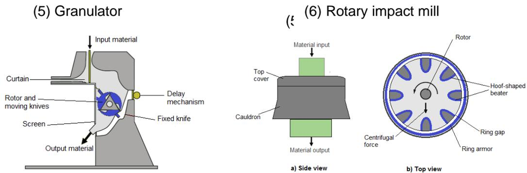
Figure 4: Schematic illustration of a granulator and a rotary impact mill [WorkSafe, 2017; BHS, 2016]
