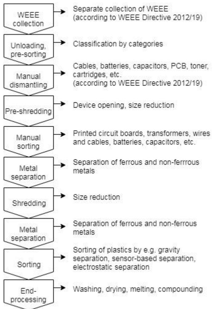
*Figure 1: Multistep mechanical separation with following sorting and end-processing according to (Batanic et al., 2018; Chagnes, 2016; Ueberschaar, Geiping, Zamzow, Flamme, & Rotter, 2017)*
