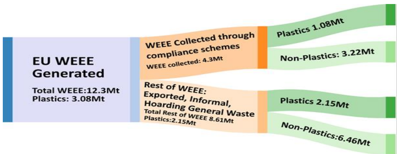
Figure 14: Plastics in WEEE streams in 2016 in EU Approximation (derived from Balde 2017, RDC 2017, Huisman et al; 2016)
